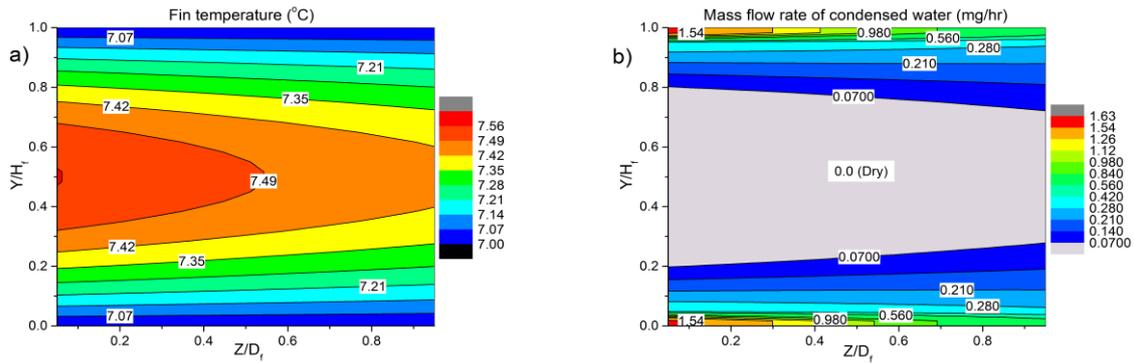
Fig. 5: (a) fin temperature profile, (b) mass flow rate of condensed water for case (II)
