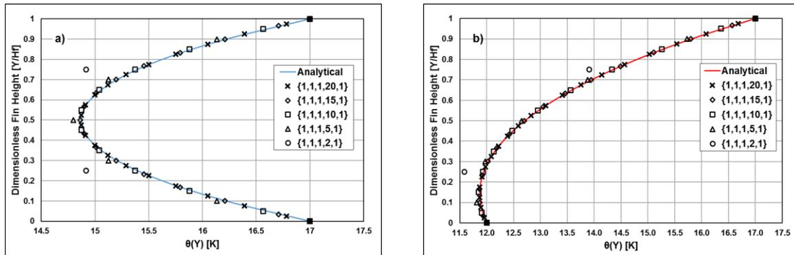
Fig. 3: V2 results for totally wet fin; (a)  $\theta(H_f) = \theta(0)$ , (b)  $\theta(H_f) = \theta(0) + 5K$
