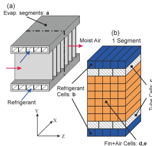
**Fig. 1:** (a) a piece of the evaporator under study, (b) schematic of the discretization in a segment of the evaporator.
