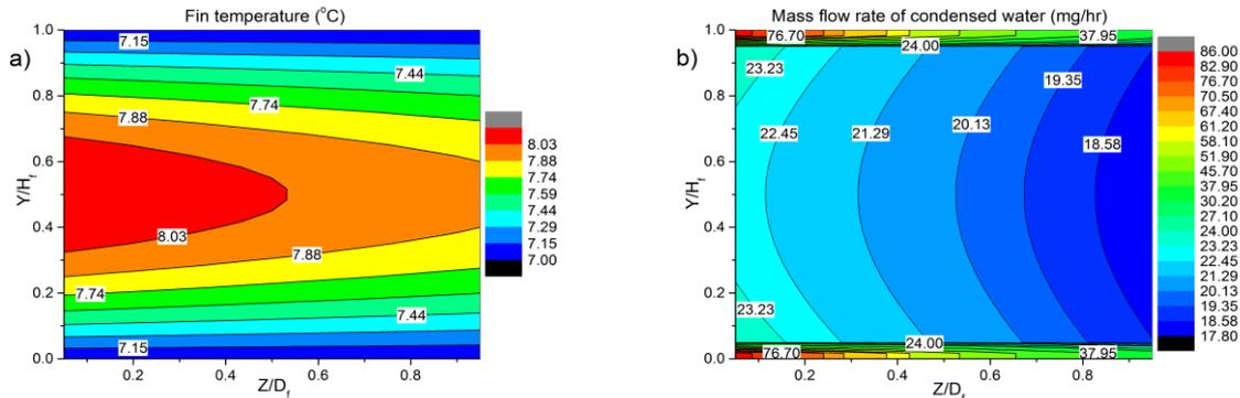
**Fig. 4:** (a) fin temperature profile, (b) mass flow rate of condensed water for case (I)
